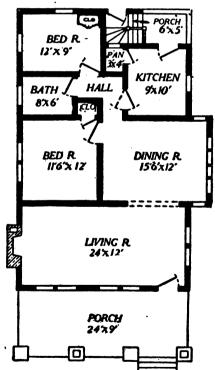
Fig. 95.—COMMUNITY I. PICTURE (IDEAL RENDERING) AND PLAN OF MILL-CUT BUNGALOW OF 5 ROOMS, BATH, AND CELLAR.
